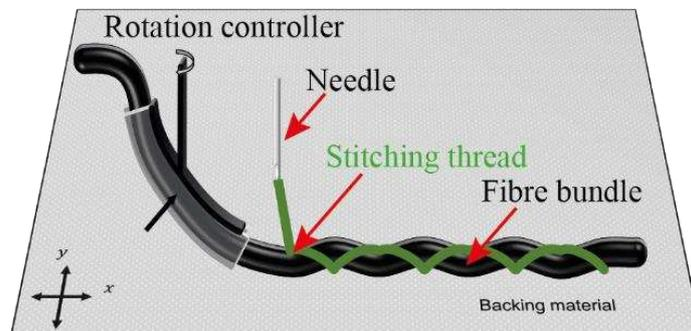
Figure 1: Principle of the TFP technique [1].
