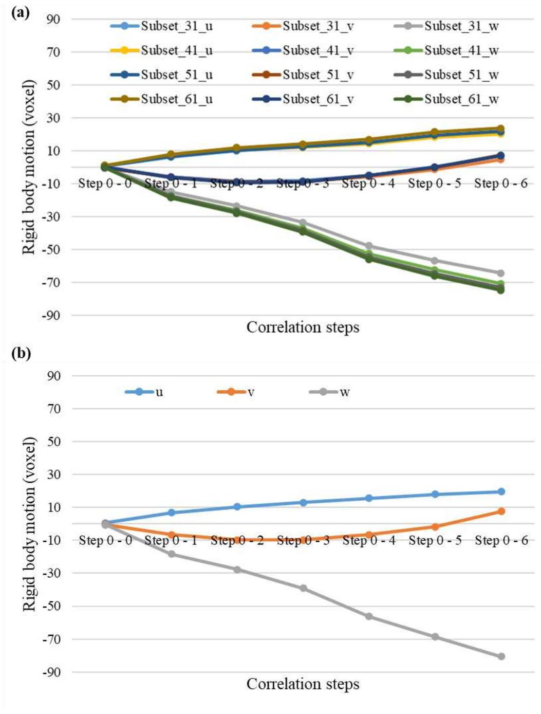
Figure 7: Three directional rigid body translations ( $u$ ,  $v$  and  $w$  along  $x$ ,  $y$  and  $z$  axes) detected from (a) Local DVC approach (for three particular subsets 31,41,51 and 61), and (b) Image processing using ImageJ.
