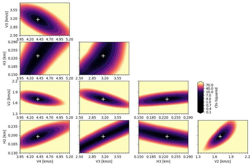
Figure S7: Individual two-dimensional slices through the  $\chi^2$  hyperspace for the five parameter grid search to identify the baseline four layer  $v_p$  model. The numerical subscripts refer to the layer position in a downwards sense from the surface; layer 1 thickness ( $H_1$ ) and velocity ( $v_1$ ) are fixed and so are not shown, layer 4 is a halfspace so  $H_4$  is not a variable.
