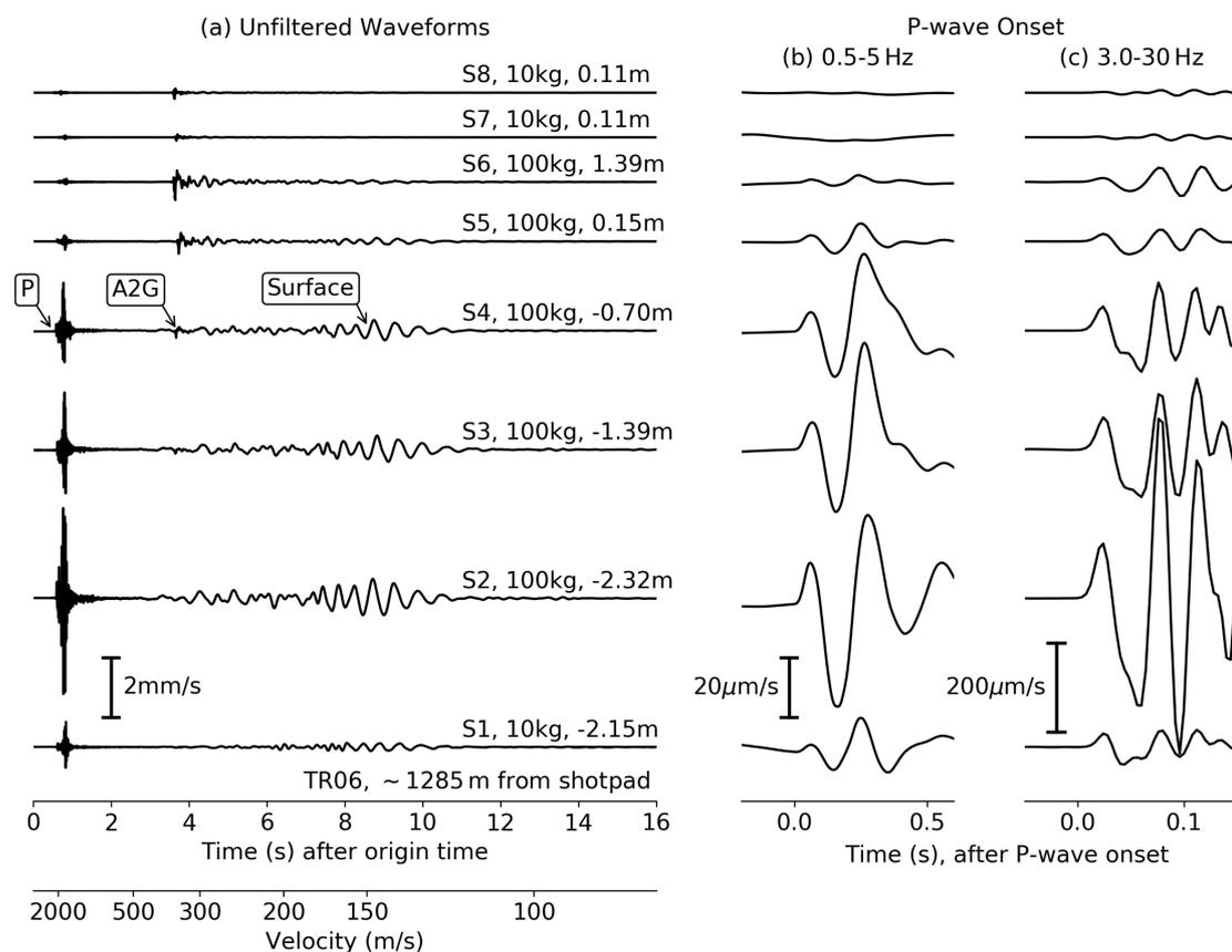
Figure 4: Velocity seismograms recorded at TR06, 1285 m from the centre of the shotpad for the eight explosions (S1 to S8). Labels to the right of panel a, showing unfiltered waveforms, indicate the explosive charge mass (kg) and HoB (m). Boxed annotations indicate the P-wave, air-to-ground coupled (A2G) and surface wave arrivals. Details of the P-wave onsets are shown in two passbands: 0.5 to 5 Hz (panel b) and 3.0 to 30 Hz (panel c).
