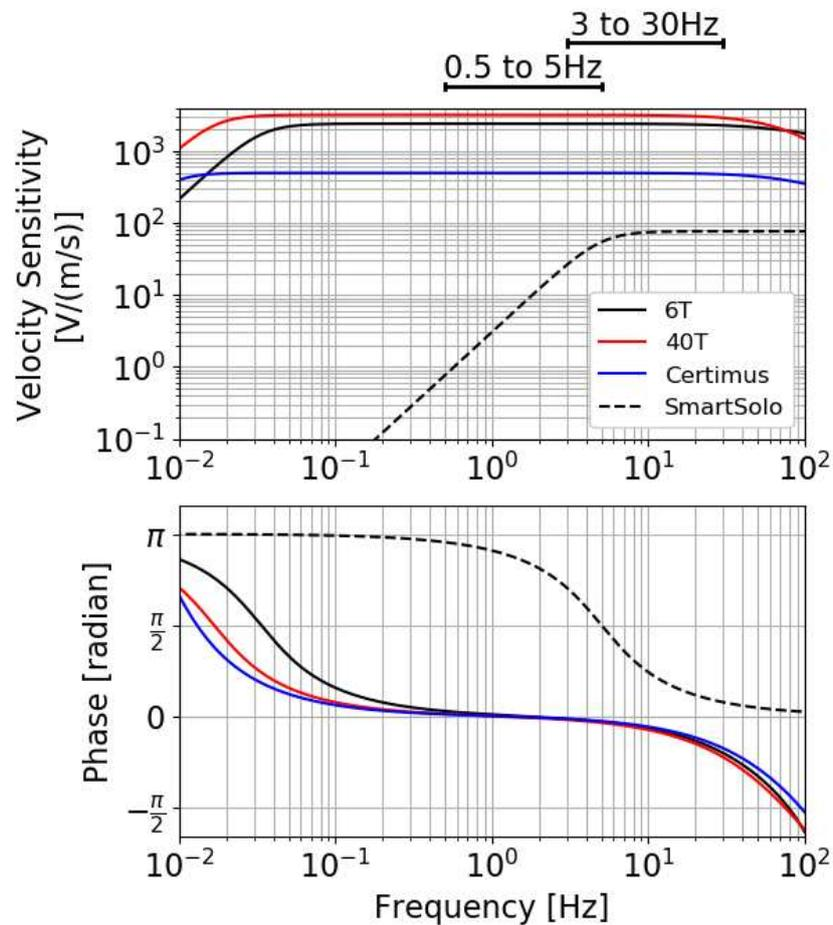
Figure S2: Instrument responses for the four types of seismic sensor deployed as part of FSCT. The geophone nodes are manufactured by SmartSolo Inc., the three broadband sensors are manufactured by Güralp Systems Ltd. The two filter passbands used in the study are provided above the plot for reference.
