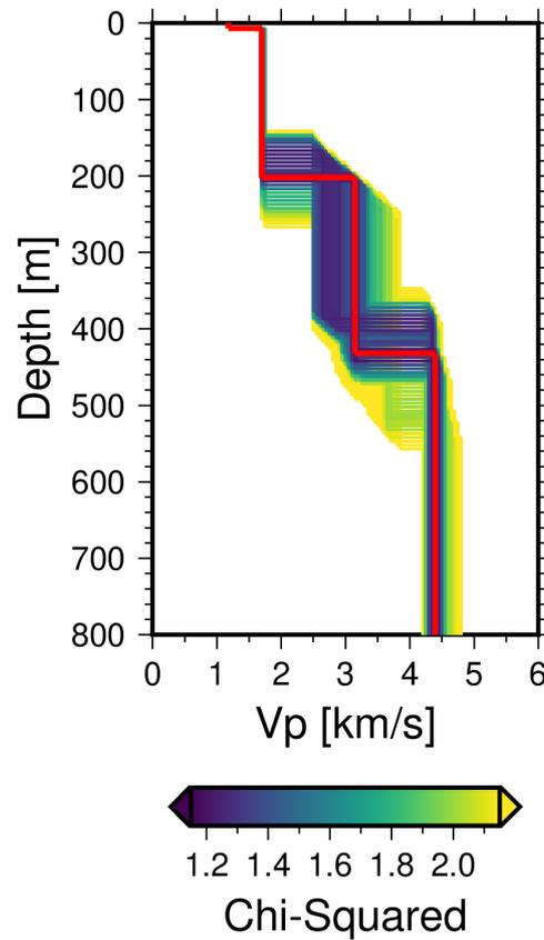
Figure S6: The 10000  $v_p$  models that exhibited the lowest  $\chi^2$  values (eq. S1) within the five parameter grid search used to identify our baseline (lowest  $\chi^2$ ) four-layer  $v_p$  model (red line). The plotted models represent  $<0.1\%$  of the considered parameter space.
