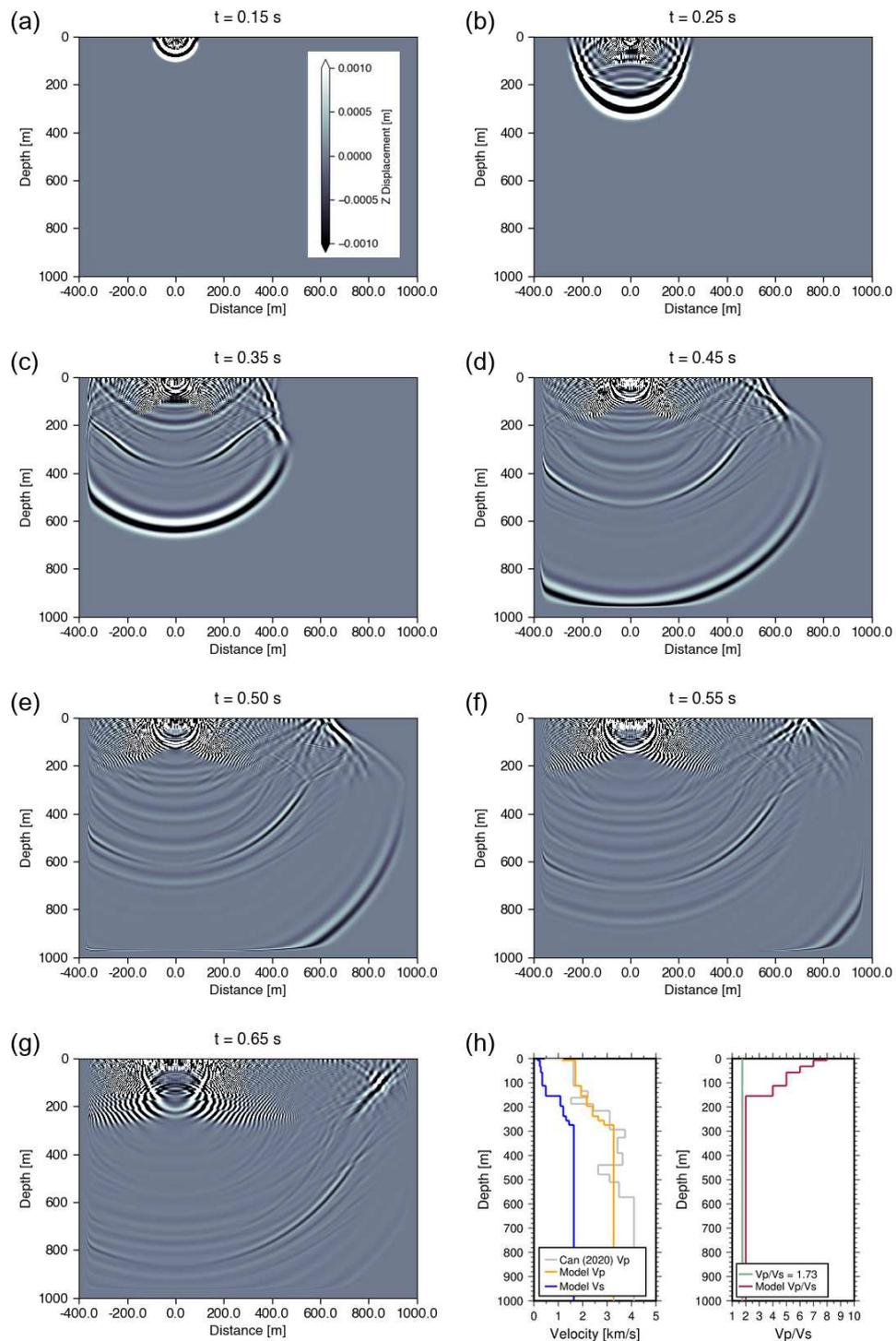
Figure S10: Snapshots from SW4 finite-difference simulations (panels a to g) showing the evolution of the vertical component seismic displacement wavefield when propagated through our preferred model.
