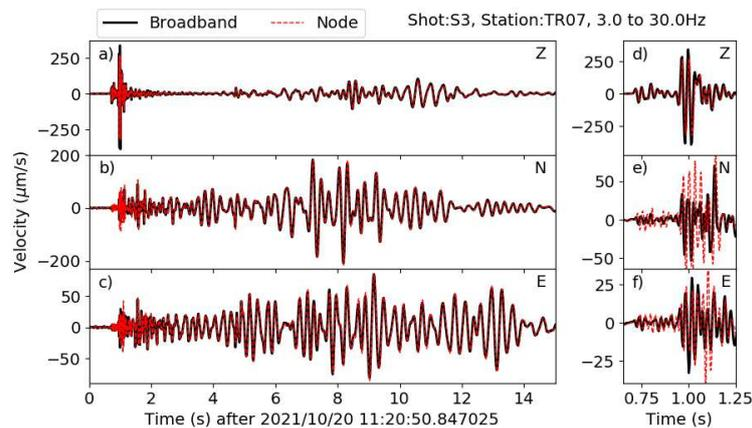
Figure S4: The same co-located broadband and geophone comparison as Fig. S3 except bandpass filtered between 3 and 30 Hz.
