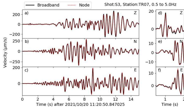
Figure S3: A comparison of three-component recordings for shot S3 on co-located broadband (Güralp Certimus) and geophone (SmartSolo) sensors. Panels a) to c) show a 15s window for the vertical (Z), north (N) and east (E) components respectively. Panels d) to f) show the detail of the *P*-wave arrival. Traces bandpass filtered between 0.5 and 5 Hz.
