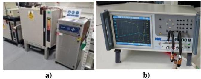
Fig. 3. Thermal degradation setup and measuring equipment: a) oven used to thermally age the coils and extractor, b) impedance analyzer WK-1J6500B.
