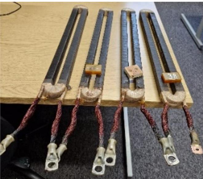
Fig. 2. Stator coils used as test hardware (C1 – C4).
