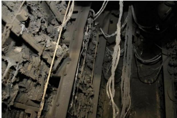
Figure 5: The remanence of battery room on MS Brim (Image courtesy of Kripos).
