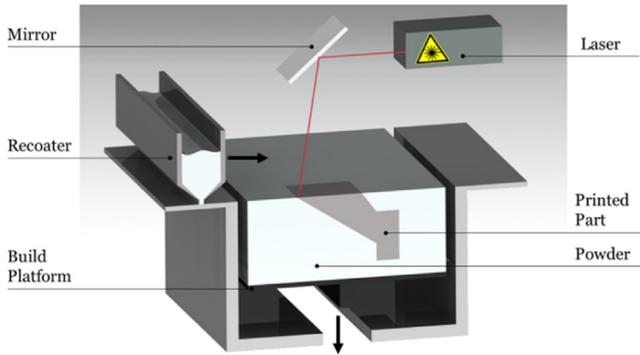
**Fig. 1.** Graphic representation of a SLS machine, showing all key components.
