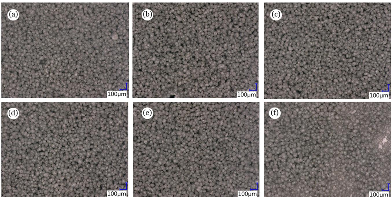
**Fig. 9.** Optical microscope images of particles from Series A: (a) Batch PA12 – 1; (b) Batch PA12 – 2; (c) Batch PA12 – 3; (d) Batch PA12 – 4; (e) Batch PA12 – 5; (f) Batch PA12 – 6.
