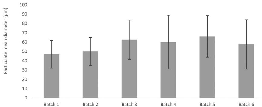
Fig. 15. PA12 particle size series A (Mean maximum and minimum from batch 1 to 6).
