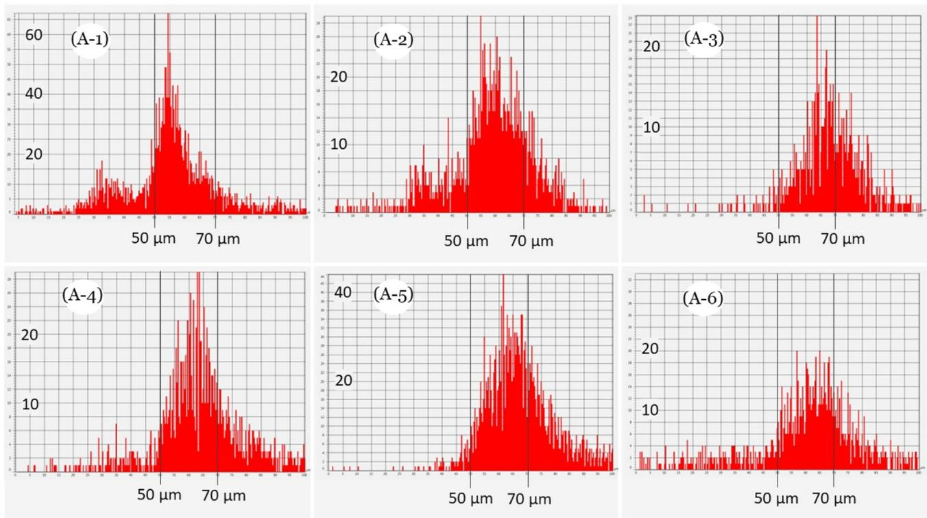
Fig. 13. Particle size distribution (Series A, for Batch 1 to 6) (X-axes represent the particle size, Y-axes represent the number of particles within each size range).
