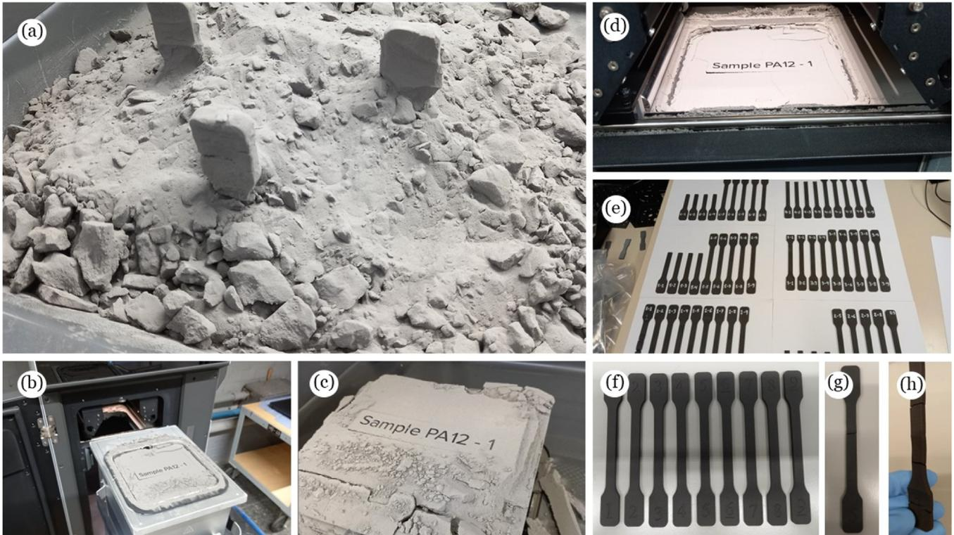
**Fig. 3.** (a) Tensile specimens in cleaning process; (b,c,d) Build box with powder and printed parts; (e,f) Printed tensile specimens; (g,h) Printed Tensile Specimen with defects.
