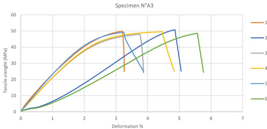
Fig. 16. Example of stress-strain diagrams that are plotted for the comparison of tensile bar number 3 across all six batches in Series A.
