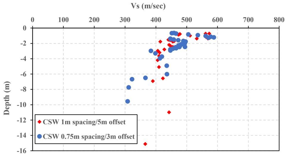
Figure 3: The results of CSW (forward shots only) for the two survey protocols.
