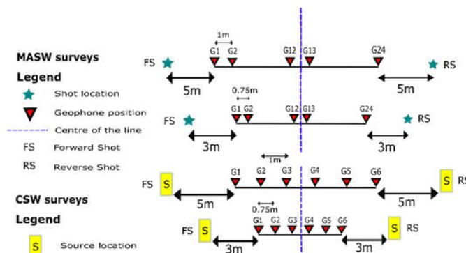
**Figure 1:** Field test protocols per method. All lines were centred between geophone G12 and geophone G13 for MASW and between G3 and G4 for CSW tests- the common mid-point represented by the blue dotted line.
