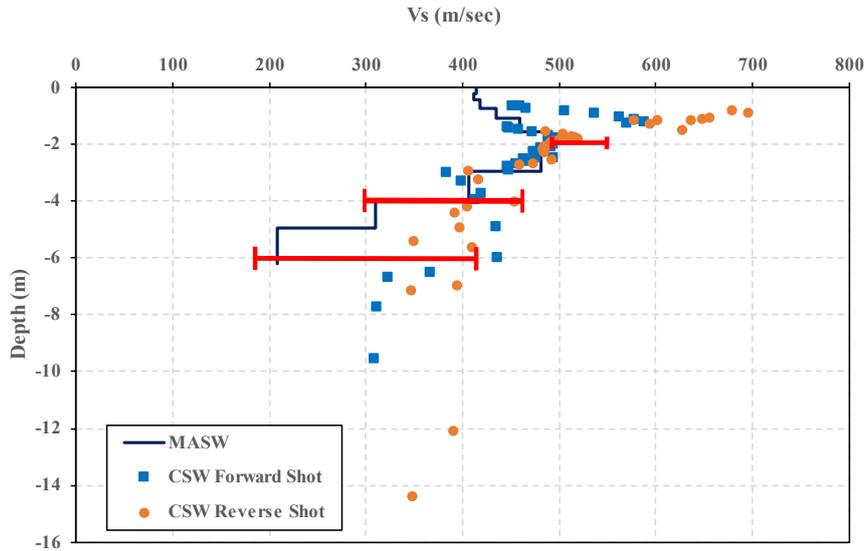
**Figure 5:** The  $V_s$  to depth profiles for both MASW and CSW surveys, for the same geophone spacing and offset location (1 m spacing, 5 m offset).
