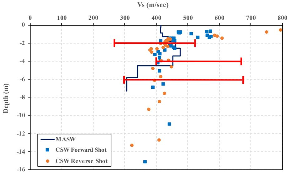
**Figure 4:** The  $V_s$  to depth profiles for both MASW and CSW surveys, for the same geophone spacing and offset location (0.75 m spacing, 3 m offset). The MASW plot is the one which best fits the CSW data.
