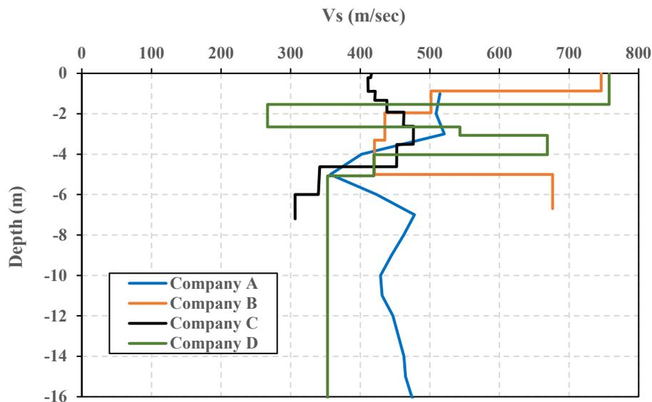
Figure 2: Example of the results of MASW for all companies - survey protocol of 0.75 m spacing/ 3 m offset.
