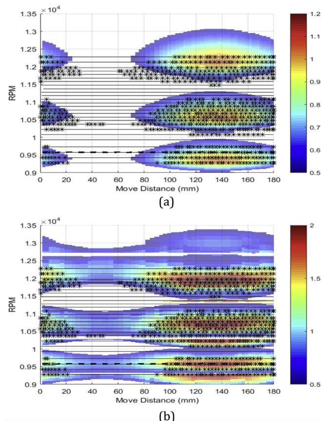
Fig. 6. Experimental results with stability roadmap, \*markers represent regions with chatter. Stability map (a) using static FRFs (b) using rotating FRFs.
