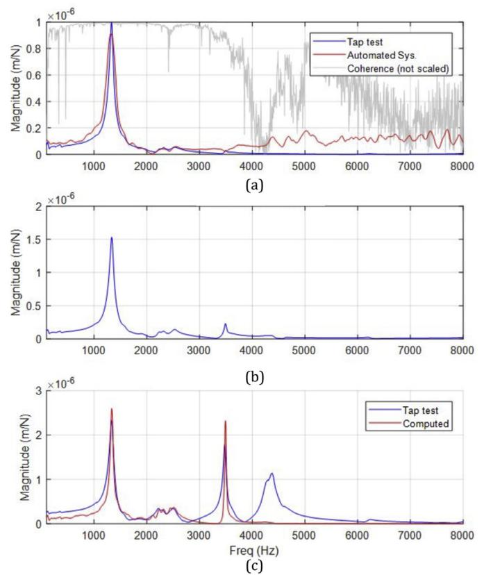
Fig. 4. Measurement at static conditions in X direction of the machine tool a)  $G_{22}$  b)  $G_{21}$  c)  $G_{11}$ .
