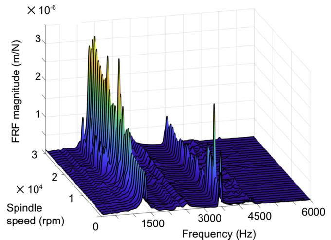
Fig. 5. Magnitude of FRF between 0–30,000 rpm.
