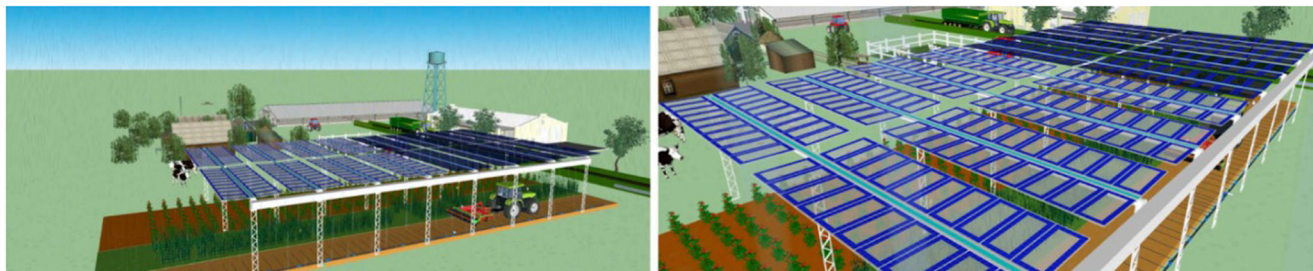
Figure 1. A schematic of the AgriPV system (left). Panels with regular and GCC glass on an agriPV system (right).
