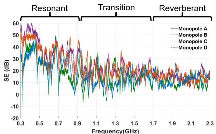
Fig. 2. SE calculated using the monopole antennas on the instrumented TL ReCo representing resonant, transition, and reverberant frequency range.
