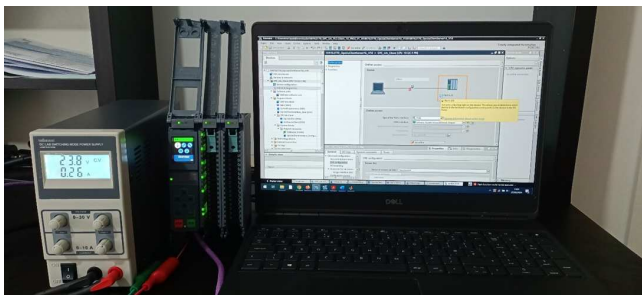
Figure 5: Siemens S7 1500 PLC connection set-up on the PC through ethernet cable.
