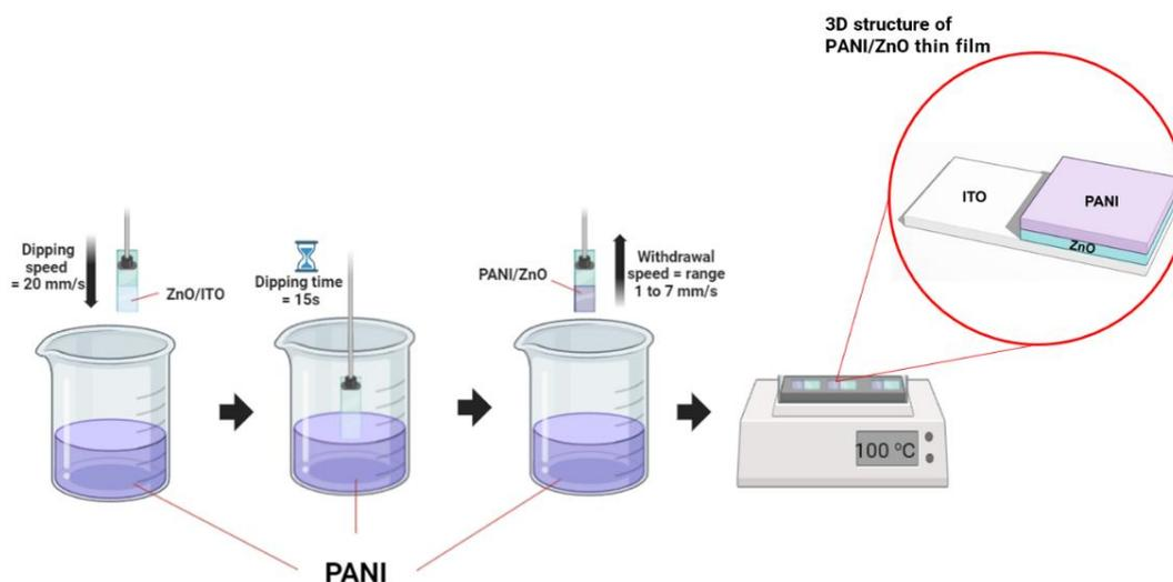
Figure 1. Dip coating method setup
