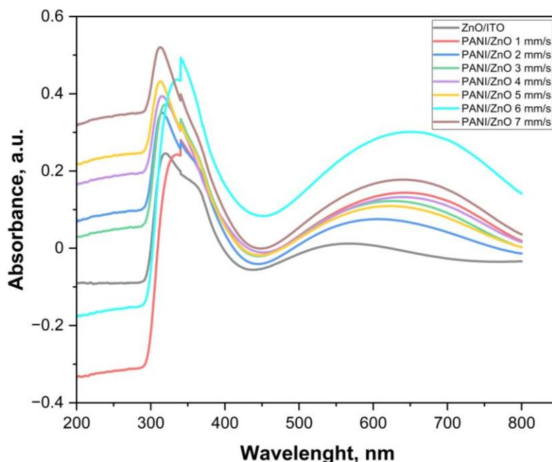
**Figure 4.** Absorption spectra for ZnO/ITO film and PANI/ZnO films at different withdrawal speeds
