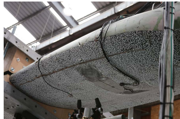
Fig. 10. Image showing blade seam failure at the overlap where the top and bottom skins of the material were bonded.
