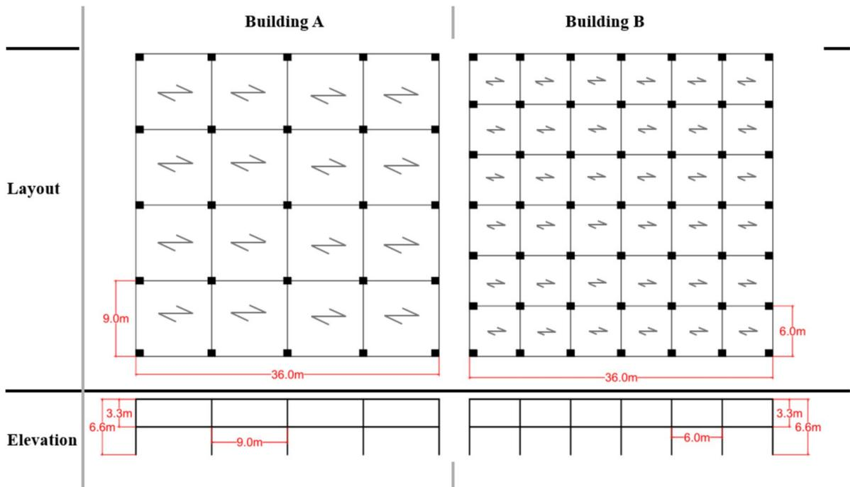
**Fig. 1** Plan and elevation views of the 9 m span (A) and 6 m span (B)—one-way load direction
