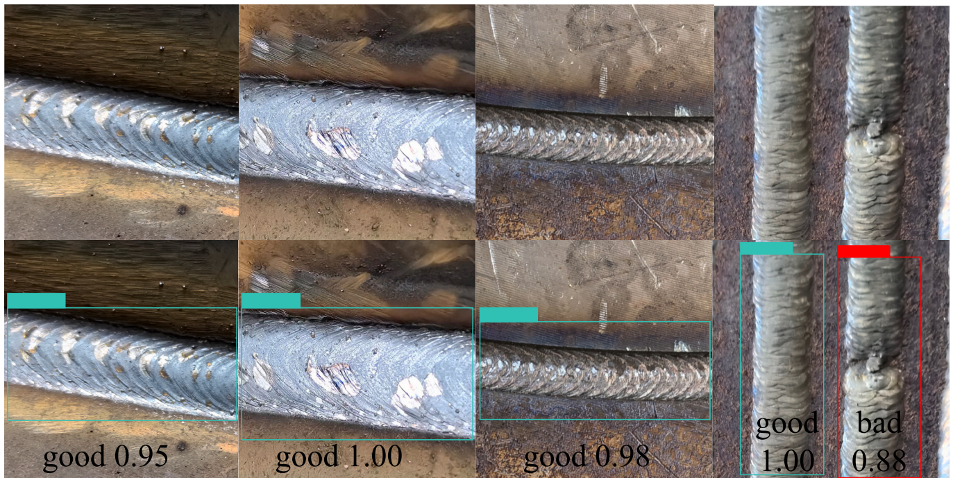
Fig. 19. Illustration of weld defect detection results in WAAM.
