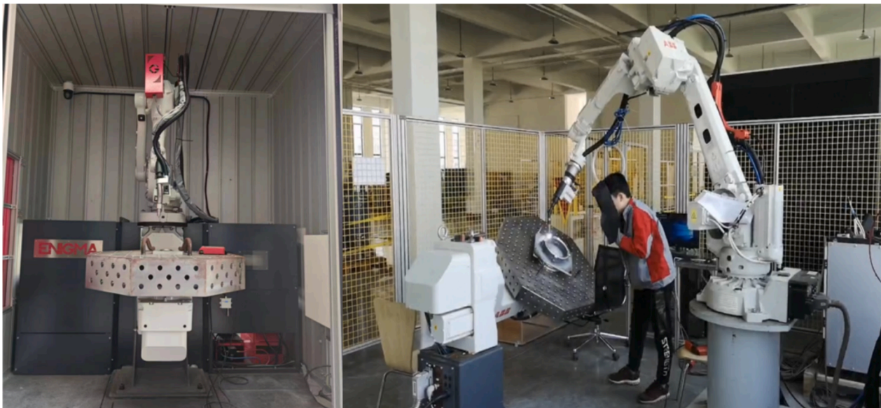
Fig. 16. Illustration of Arc Additive Manufacturing System ArcMan S1 Adv.
