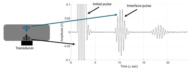
**Figure 3:** Initial pulse and reflected ultrasonic waves from the boundaries of the workpiece.
