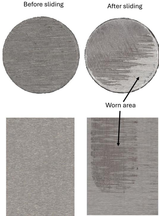
**Figure 4:** Fresh and worn pin and workpiece scanned by a 3D optical profilometer (Alicona Infinite Focus SL).
