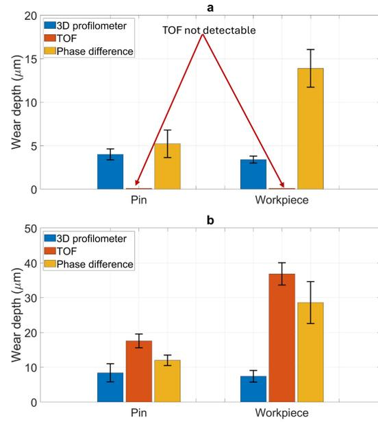
**Figure 8:** Wear depth measured with a 3D optical profilometer, TOF and phase difference of the pin and workpiece after: (a) 5m; (b) 200m sliding.
