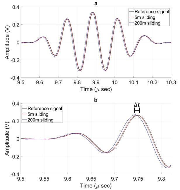
**Figure 5:** A comparison of the time domain reflected waves before sliding, after 5m and 200m sliding of the pin: (a) full reflection (b) zoomed in.
