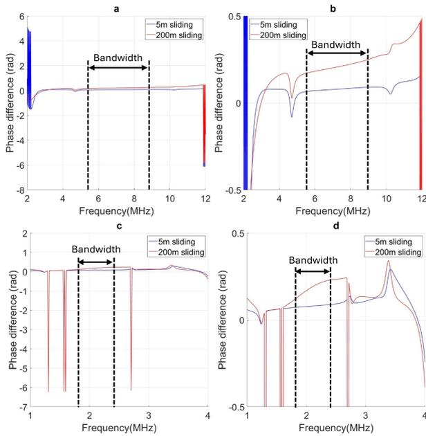
**Figure 7:** The phase difference of FFT transforms of reflected ultrasonic waves at the 5m and 200m sliding: (a) pin; (b) y-axis zoomed-in of the pin; (c) workpiece; (d) y-axis zoomed-in of the workpiece.
