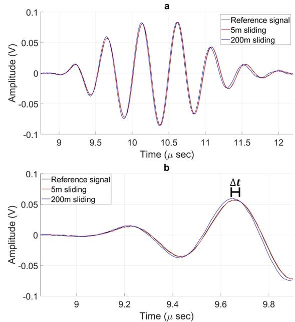
**Figure 6:** A comparison of the time domain reflected waves before sliding, after 5m and 200m sliding of the workpiece: (a) full reflection; (b) zoomed in.
