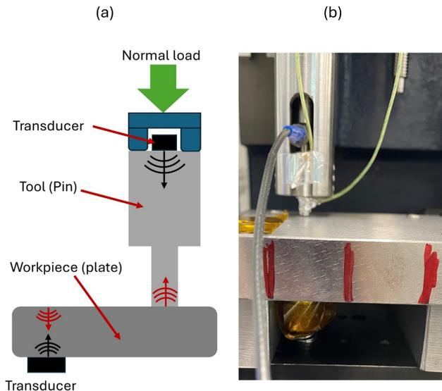
**Figure 1:** Experimental set-up: (a) schematic diagram; (b) experimental apparatus.
