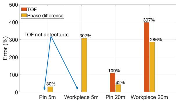
**Figure 9:** Percentage error of the TOF and phase difference of the wear depth in the pin and workpiece.
