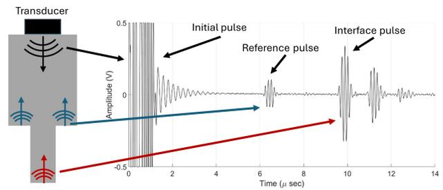
**Figure 2:** Initial pulse and reflected ultrasonic waves from the boundaries of the pin.
