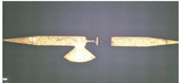
Fig. 11. Fabricated single bond wire with impedance compensation.
