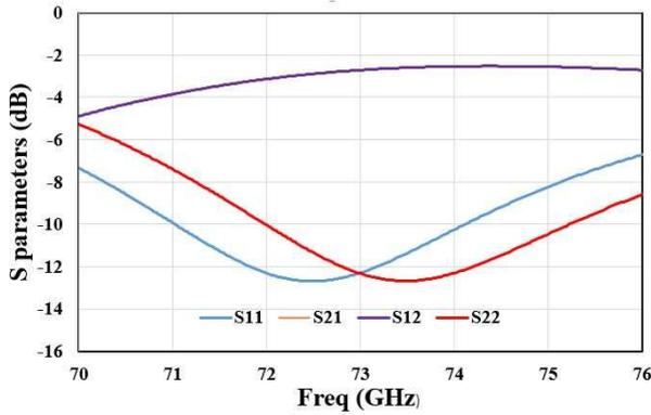
Fig. 7. Simulated S parameters of the compensation circuit.
