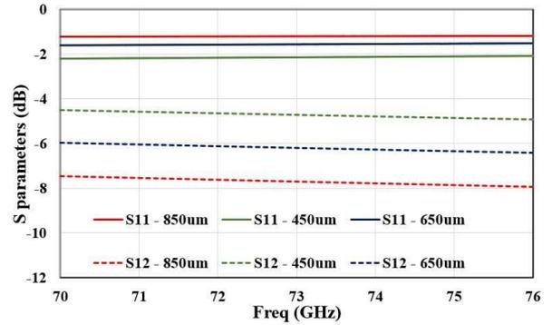
Fig. 4. S parameter results of the bond-wire interconnection with the change in length.
