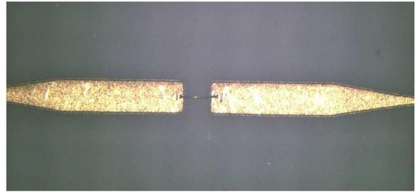
Fig. 9. Fabricated single bond wire.
