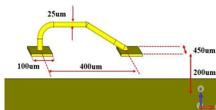
Fig. 1 Simulation model of the bond wire.
