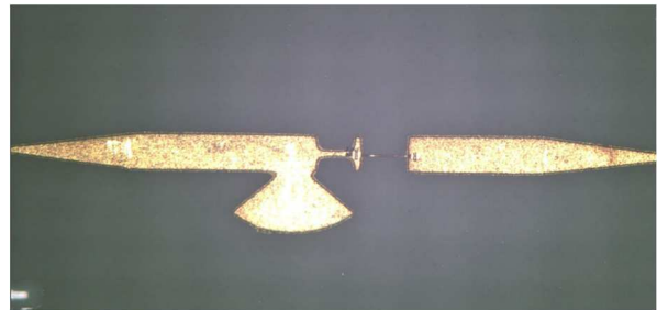
Fig. 11. Fabricated single bond wire with impedance compensation.
