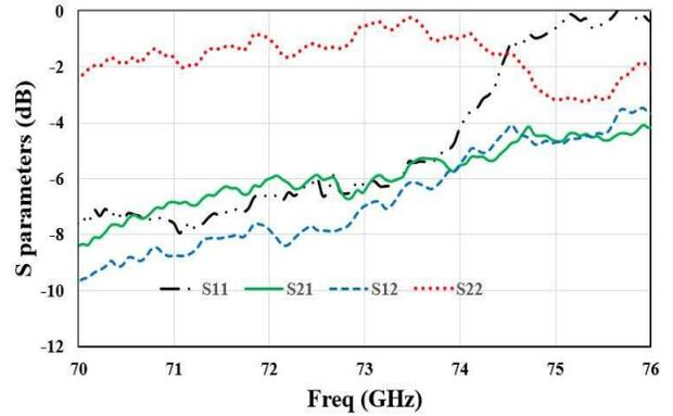
Fig. 10. Measured S parameters of the single bond wire.
