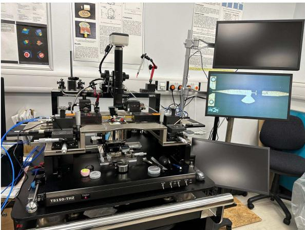
Fig. 8. Probe station for S parameter measurement.
