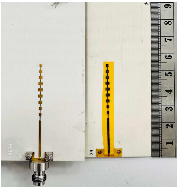
Fig. 6. Fabricated etched series fed antenna array and AJP on Kapton array.
