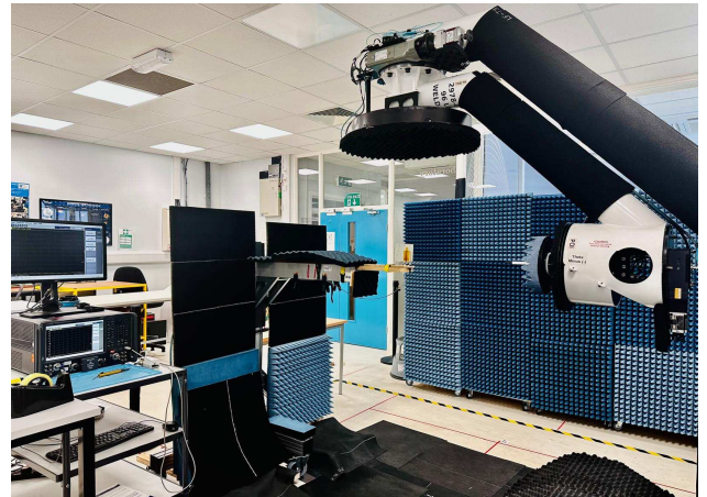
Fig. 7. NSI spherical antenna measurement system for radiation pattern measurement [18].
