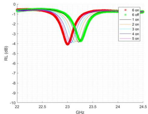
Fig. 11. De-embedded measured 23 GHz PCB six cold FET switched SIW RL as function of switch state.
