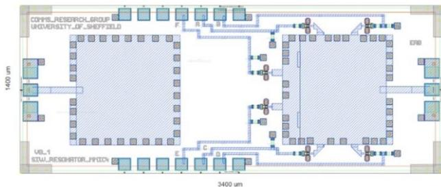
Fig. 3. MMIC layout of proposed 73 GHz SIWs: fixed SIW (left) and switched cold-FET tunable SIW (right).
