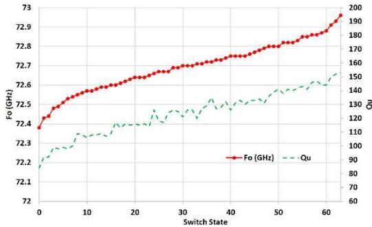
Fig. 7. ADS simulation of cold FET switched SIW on GaAs – tuning steps and  $Q_u$  over all switch states.
