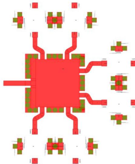
Fig. 4. PCB artwork of 23 GHz cold FET tuned SIW (FETs not shown).
