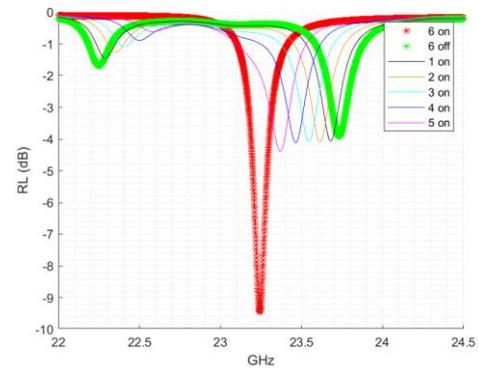
Fig. 10. ADS simulation of the cold FET switched 23 GHz SIW RL as function of selected switch state.
