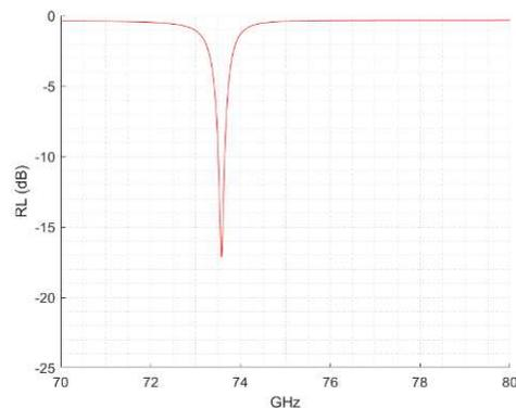
Fig. 5. ADS simulation of RL for simple fixed frequency SIW on GaAs.
