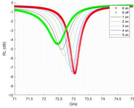
Fig. 6. ADS simulation of RL for cold FET switched SIW on GaAs.
