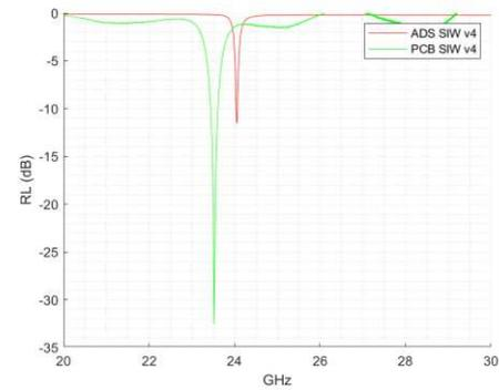
Fig. 9. Comparison of measured (de-embedded) fixed SIW to ADS model.
