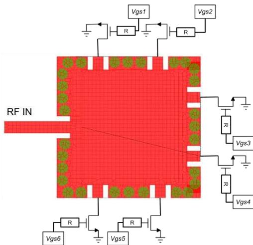
Fig. 2. SIW with vias removed and cold FETs added to TAPs.
