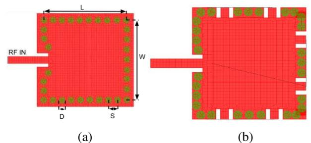
Fig. 1. Layout of a simple SIW: a) key dimensions, b) vias removed where TAPs added.
