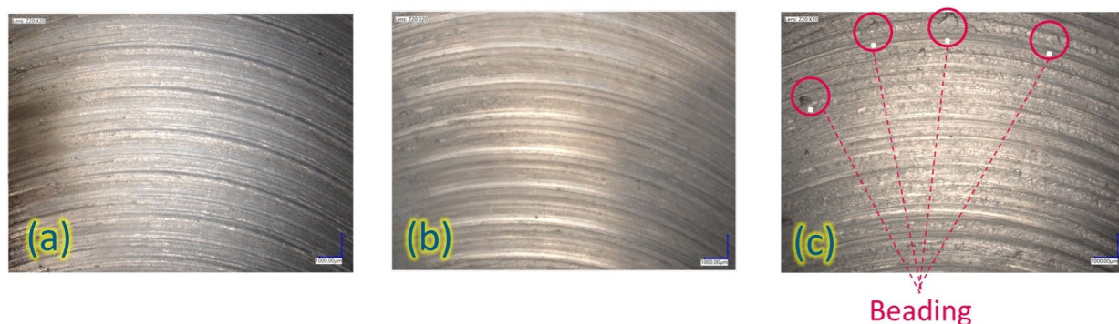
Figure 11. Upper surface topographies of specimens: (a) Exp-1, (b) Exp-2, and (c) Exp-3.
