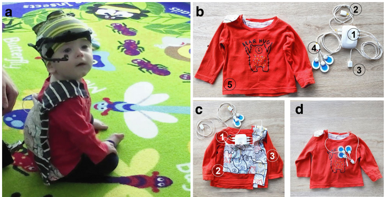
Fig. 2. The wearable body sensor. (a) Example of a 9-months-old infant wearing the head-mounted eye tracker with the body sensors. (b) The Biosignals Plux wearable sensors: 1—the data recording hub; 2—the light sensor; 3—the acceleration sensor; 4—the ECG sensor with the Ambu blue electrodes (Ambu, Copenhagen, Denmark) attached; 5—the custom-made shirt. (c) The back view of the shirt showing how the sensors were embedded: 1—eyelet, which allows the ECG and Acc sensors to be brought from the back to the front and positioned on the left side of the chest; 2—the back pocket, which holds the data recording hub; 3—the shirt closes at the back via hook and loop. (d) Front view of the shirt with the sensors embedded, illustrating the location of the ECG sensor.
