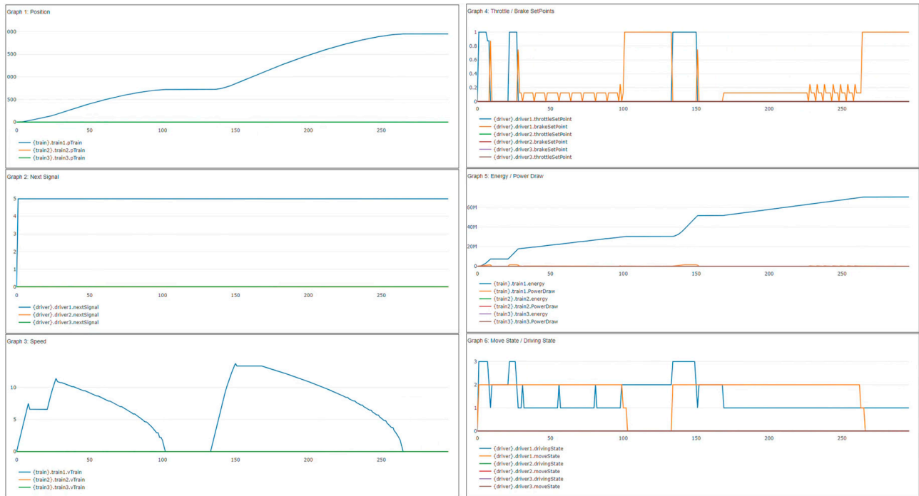
Figure 11. Screenshot of the INTO-CPS Application showing live plots of a single train stopping at two stations.
