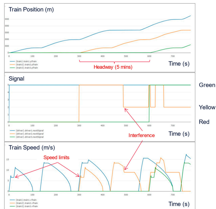
Figure 12. Annotated graphs showing train position, signal state, and speed; notice the interference as the second train catches up to the first and is on a yellow signal.
