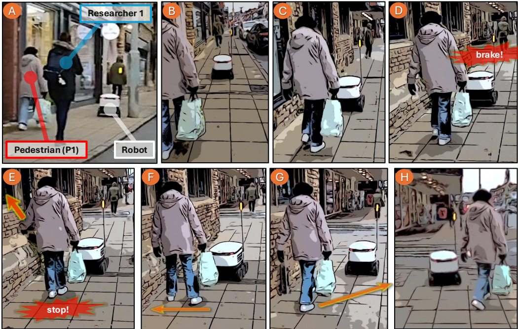
Fig. 2. Following and Overtaking. A pedestrian (P1) is following a delivery robot (A). The delivery robot drives in a somewhat meandering way, gradually arriving at a more leftwards position laterally on the pavement and having slowed somewhat, closing the distance between the pedestrian and the robot (B, C). The robot brakes abruptly (D), causing the pedestrian to also stop immediately (E), which then leads to them sidestepping (F), perhaps to get around the now-stopped robot. However the robot starts driving again (G) while the pedestrian moves rightwards to overtake the robot, heading towards the road crossing (H).
