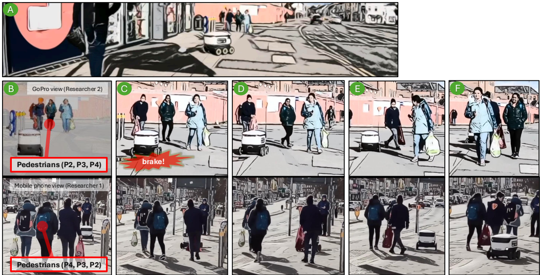
Fig. 3. Using a ‘Bulge’ to Pass By. A group of three pedestrians (P2, P3, P4) are walking towards a robot that is also turning towards them on a wide pavement in front of a grocery shop (A). As the pedestrians continue their walking trajectory, the robot is headed in their direction (B). As their paths intersect, the robot brakes abruptly (C) while the group arcs around the robot (C-F) with P2 lagging slightly behind the others. During this arc, the robot continues on its way (E-F).
