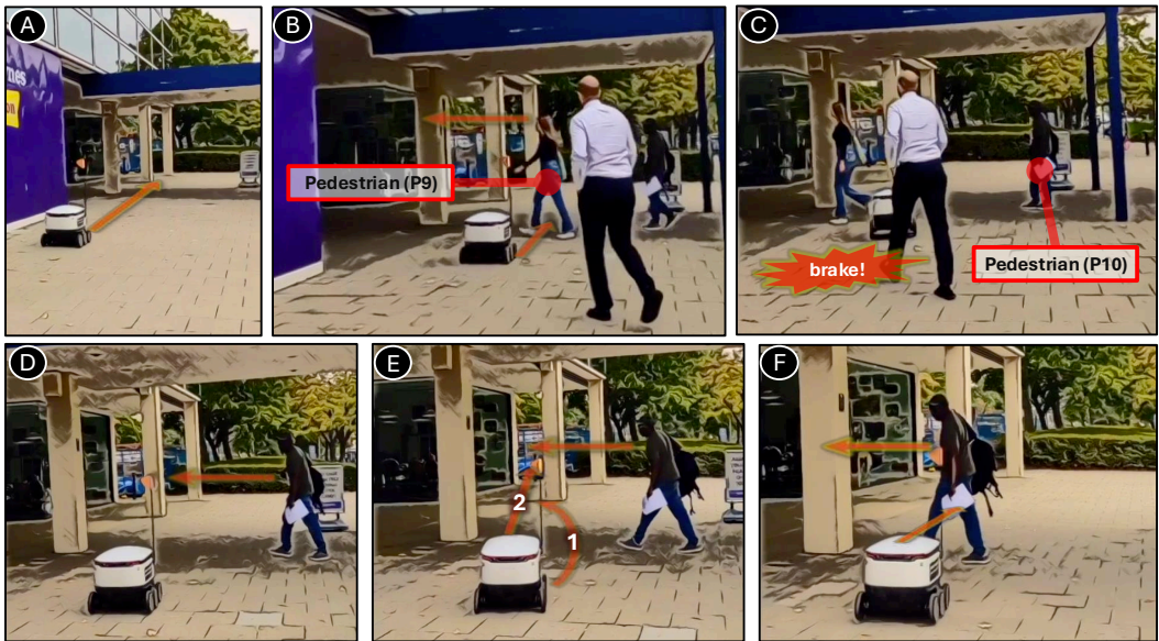
Fig. 7. Dealing with an Intersection. A robot crosses an entrance to a shopping centre (A) while three pedestrians approach the entrance from different directions. P9 and P10 have trajectories that are orthogonal to the robot's (B-C); P9 crosses the path of the robot (B) and the robot brakes forcefully just after the intersection of paths (C). Just before the robot brakes, P10 pauses momentarily while looking towards it. After brief hesitation, P10 then makes a move towards the entrance (D). Shortly after, the robot turns (E-1) and then begins to drive towards the emerging trajectory of P10 (E-2). P10 clears the space while the robot continues its driving (F).
