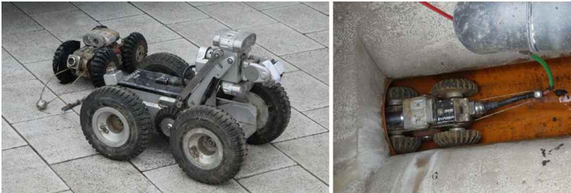
Figure 4.1 Typical CCTV inspection crawlers showing differing sizes (left) and tethered crawler entering pipe from a benched manhole (right). (Courtesy Will Shepherd).
