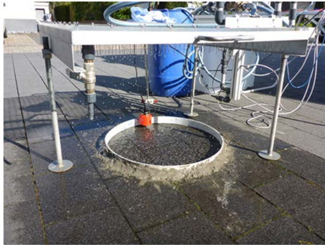
Figure 4.18 In-situ test for infiltration of a permeable pavement in Germany. (Courtesy F. Boogaard).
