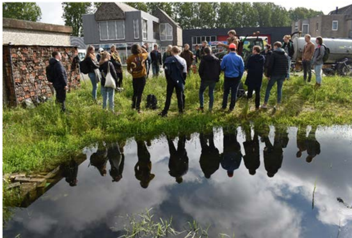
Figure 4.20 Example of hydraulic test on a swale with the full-scale test in Groningen (tank truck on the right), measurements by loggers in the swale and hand measurement of students from Hanze Applied University of Groningen. (Courtesy F. Boogaard).
