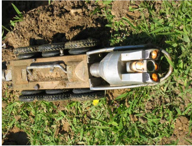
Figure 4.21 Picture of a mobile vision-based inspection system showing the lights (in front), the camera (between the lights), the swivel head (camera + lights), and the motorized crawlers (left part). (Courtesy F. Cherqui).
