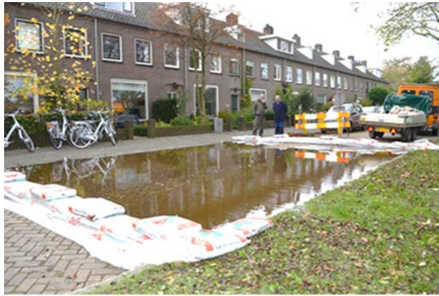
Figure 4.19 Full-scale infiltration test (FSIT) where a large part of permeable pavement is flooded is applied in the Netherlands. (Courtesy F. Boogaard).
