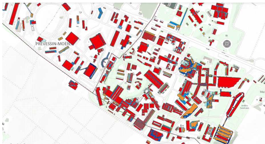
Figure 8. Map of CERN buildings. Rooftops that are suitable for PV installation in respect to their received solar irradiation are shown in red (very suitable) and yellow (suitable). In addition other areas like e.g., parking lots could also be covered by PV-panelled roofs. Reproduced with permission from [113].
