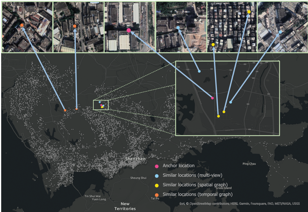
Figure 5. The results of similar location (cell tower) search. A selected anchor point (pink) is presented along with the two most similar locations using the embedding fusing three views (blue), fusing transition and spatial views (yellow), and fusing transition and temporal views (orange).
