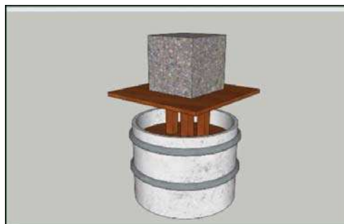
Fig. 2. Loading arrangement used for curing stabilized peaty clay samples
