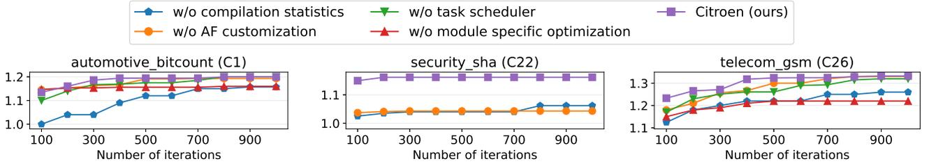
Figure 9: Ablation study on different benchmarks. The y-axis is the speedup relative to -O3. `security_sha` only owns one hot module, thus “task scheduler” and “module specific optimization” are not applicable to such single-module cases.
