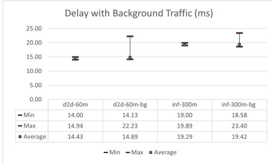
Fig. 10. The impact of background traffic on GOOSE flow delay variation in a single-cell network with D2D and infrastructure communication.
