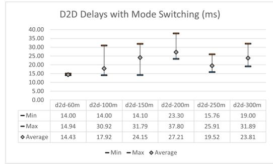
Fig. 7. Average GOOSE flow delay for D2D communication with mode switching in a single-cell network.
