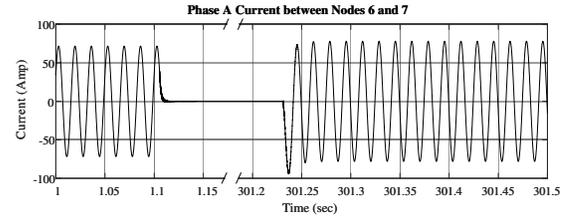
Fig. 4. Phase A current between node 6 and 7 in the IEEE 33-bus distribution test system for the FLISR case under study.
