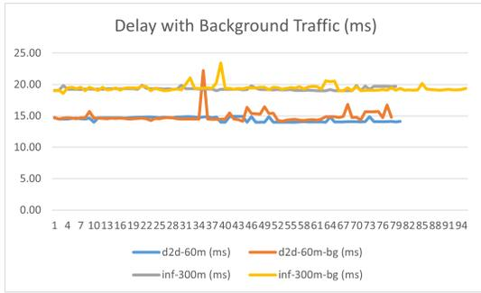
Fig. 9. The impact of background traffic on GOOSE flow delay in a single-cell network with D2D and infrastructure communication
