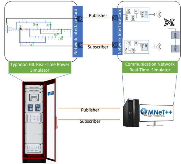
Fig. 1. Co-simulator architecture for simulating LTE networks in smart distribution systems
