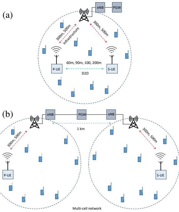
Fig. 6. LTE network configurations: a) Scenarios 1 and 2, b) Scenarios 3.
