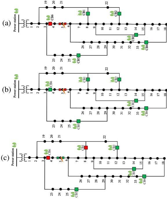
Fig. 3. IEEE 33-bus distribution test system: (a) A fault occurs at node 5, (b) Circuit breaker CB6 opens and clears the fault, (c) Operators in the control centre open the sectionalizing switches at both sides of node 5 and close the circuit breakers CB1 and CB6 to restore power to unfaulty parts of the distribution system.
