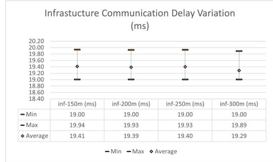
Fig. 8. Average GOOSE flow delay for infrastructure communication in a single-cell network.
