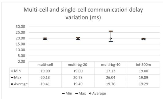
Fig. 11. The GOOSE flow delay in single-cell and multi-cell networks with and without background traffic.
