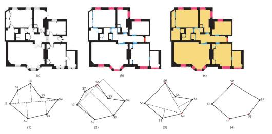
Figure 3 (a) the input floor plan image (b) recognized building elements including windows (pink), doors (blue) and entrances (red) (c) detected room regions
