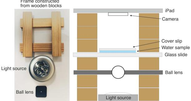
Frame constructed from wooden blocks
