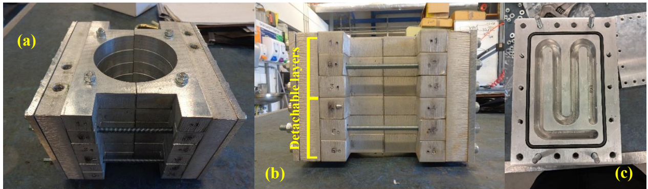
191 Fig. 3. (a) Freezing jacket, (b) front-view of freezing jacket with detachable layers, and (c) 192 internal circuit for coolant circulation.
