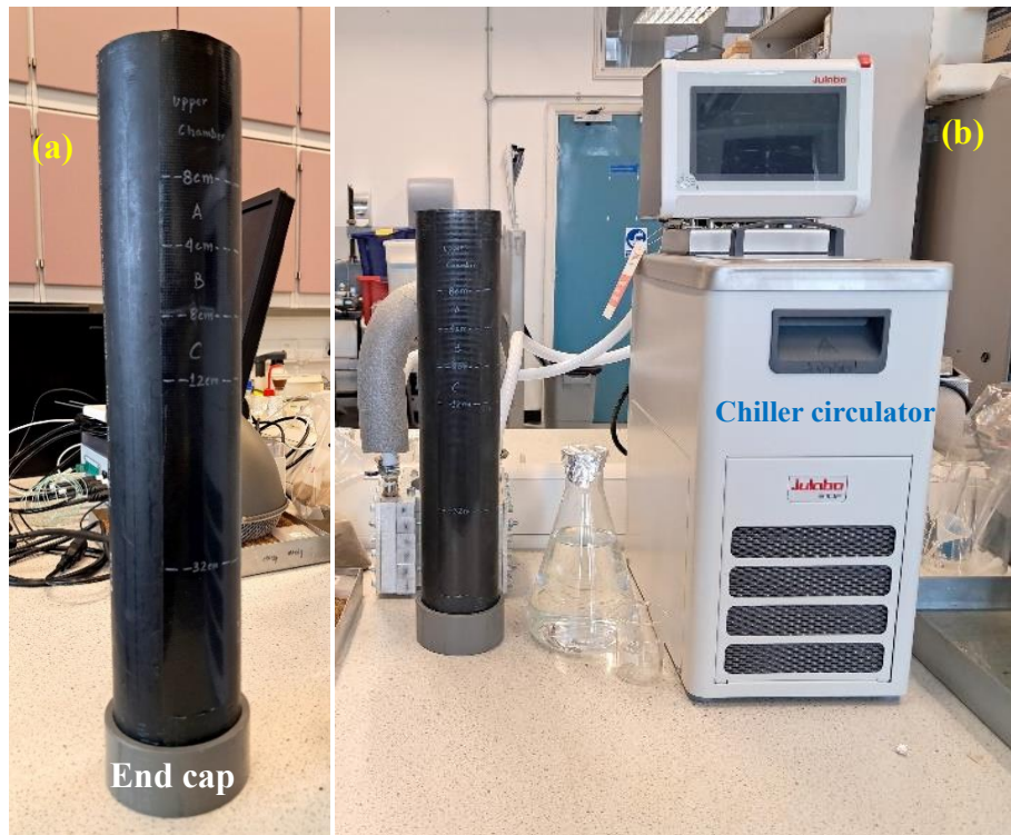
171 Fig. 2. (a) UPVC column used for the FT experiments, and (b) laboratory set up for FT 172 studies.
