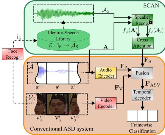
Figure 2. SCAN is shown in the top box which leverages speaker-specific information for framewise comparison of reference speech and input audio signal via cross-attention. The bottom box shows a typical ASD architectural design (baseline). Dotted connections represent non-end-to-end passages in the framework.
