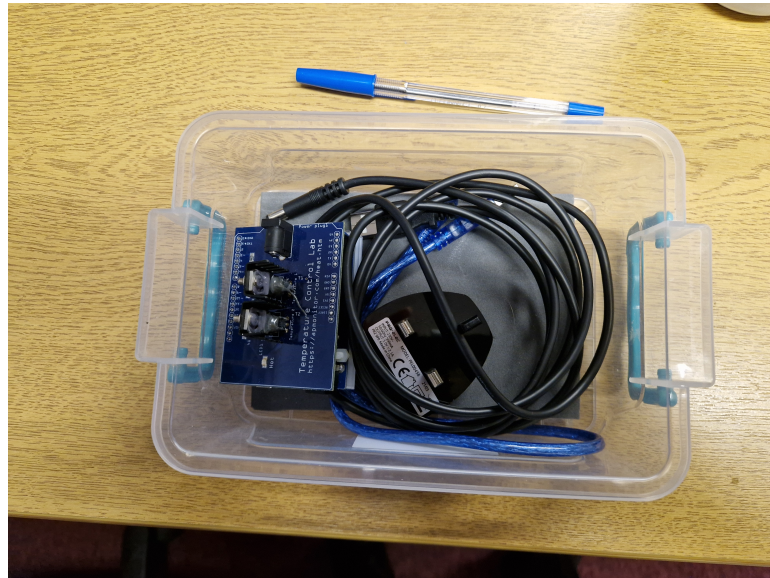
Figure 1. Example of a cheap take-home kit (two heaters) in a small sandwich box .
