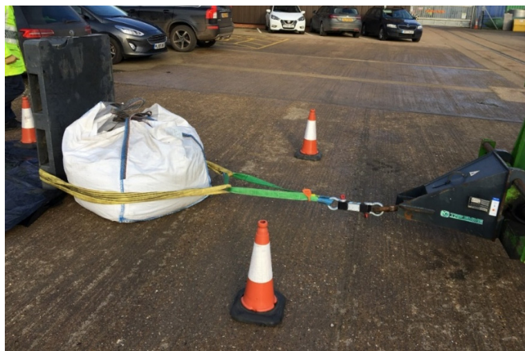
Figure 6. Single bulk bag subject to lateral tensile force during testing of surface C.
