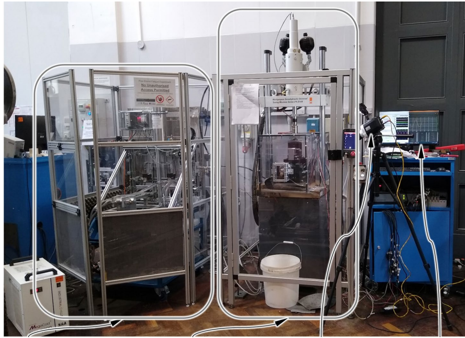
Internal water pressure loading hydraulic system LFV-25-ME fatigue machine with bending apparatus High-speed camera PC running LabView and LFV-25-ME software
