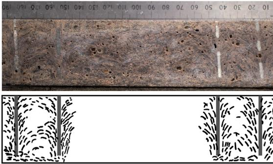
**Fig. 11** Fibre distribution between outer and inner electrodes (M-0.75%CF series)
