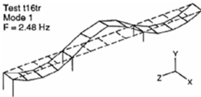
FIGURE 2 | First mode of a highway bridge in its undamaged condition, as identified from experimental measurements.
