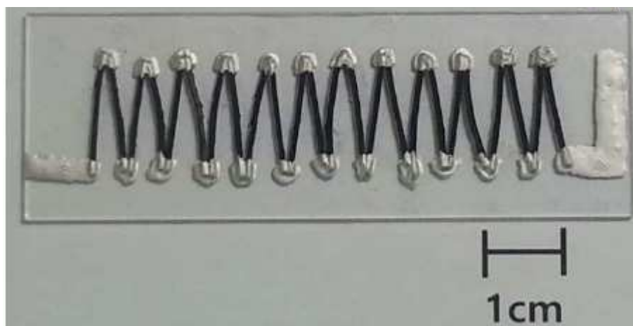
1250 Fig. 43. Photo of the organic fibre-based TE generator sewn onto a PDMS substrate [159]. 1251
