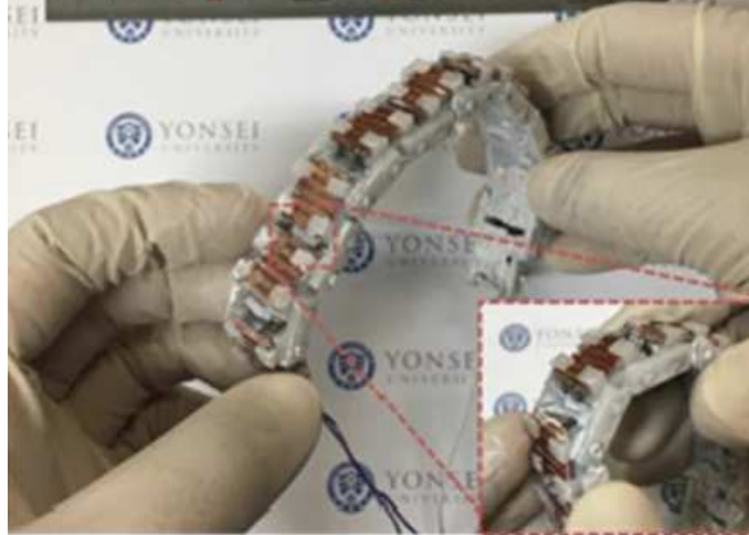
Fig. 10. The designed flexible TE module consisting a flexible holder [78].
