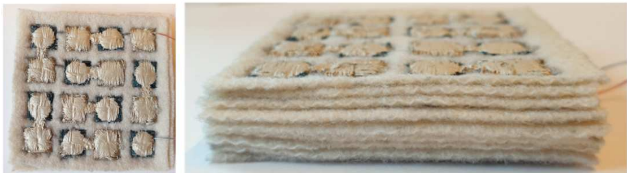
1068 1069 Fig. 35. Photos of the embroidered thread-based thermopile [143].
