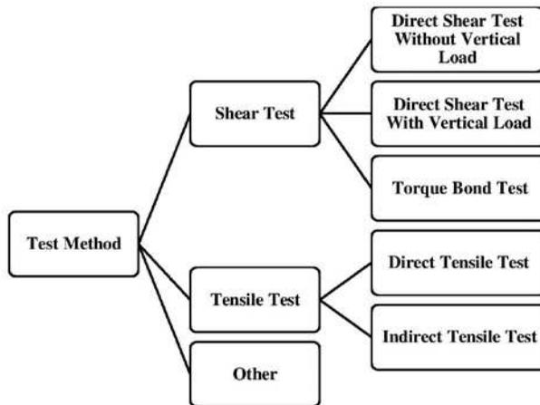
Figure 2. Types of test methods for interface bonding.
