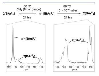
**Figure 9.** Sequential reaction of crystalline  $2[BAr^{F}_{4}]$  with CH<sub>4</sub> (8 bar gauge) and then application of a high vacuum. Insets show  ${}^{31}P\{{}^{1}H\}$  SSNMR spectra of each reaction.
