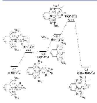
**Figure 10.** Periodic DFT free energy profile (kcal/mol) computed at 80 °C for methane loss from  $\alpha$ -1[BAr<sup>F</sup><sub>4</sub>] to give 2<sup>+</sup> $(\alpha\alpha$ -1[BAr<sup>F</sup><sub>4</sub>]. Structures show key distances (Å) in the reacting cation; intermediate and transition state labels omit the unit cell designation for simplicity. Method: PBE-D3/DZVP-MOLOPT-SR-GTH/GTH-PBE/700 Ry cutoff.
