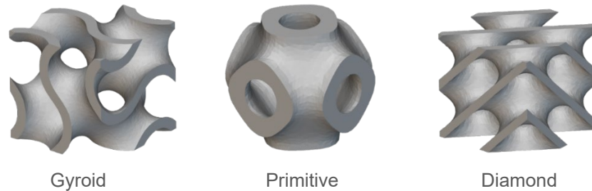
Figure 1. Examples of a unit cell of each type of scaffold included in this study.
