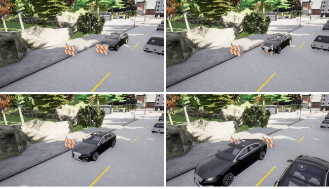
Fig. 2. Sequence of frames from replaying “Scenario 8”, the most flaky scenario found in CARLA. The ego vehicle passes through the street barrier in one of the scenarios due to a software bug.
