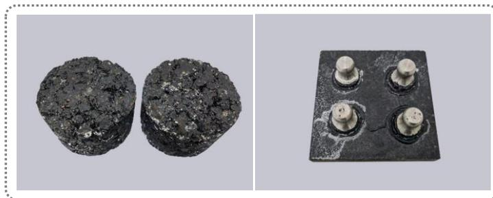
**Figure 12 The phenomenon of "salt crystallization"**
