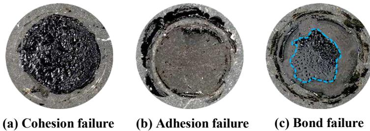
Figure 3 Failure types of BBS test
