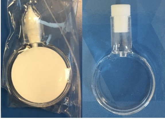
FIG. 1. Left: The sealed cuvette with ^{176}\text{Yb}_2\text{O}_3 powder. Right: An empty quartz cuvette with its polyethylene cap.
