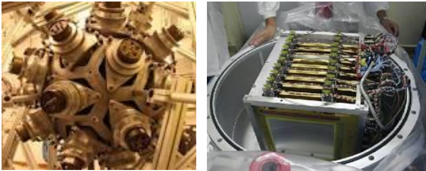
Fig. 2 Left panel the Total Absorption Calorimeter (TAC) , Right panel Parallel Plate Avalanche Chamber PPAC
