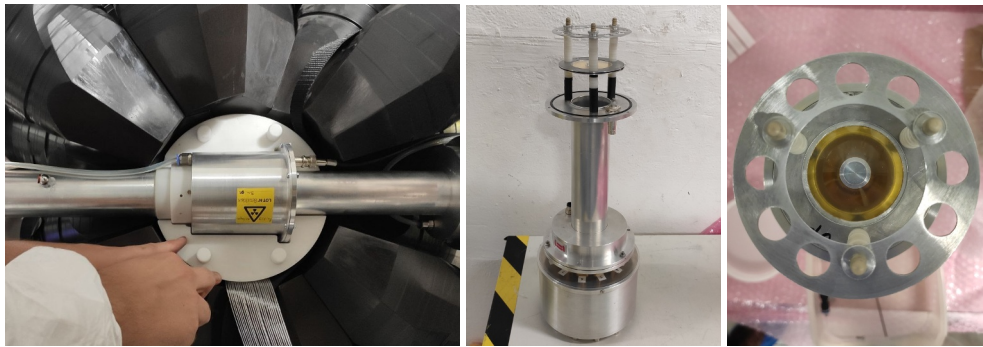
Figure 3. Photographs of the experimental setup of the ^{239}\text{Pu} measurement at n_TOF. Left: mounting of the Li-doped polyethylene neutron absorber surrounding the FFD, located at the center of the TAC. Middle: modified version of the dummy fission chamber with the thick plutonium sample for the second experimental configuration, before mounting inside the TAC. Right: top view of the ^{239}\text{Pu} thick sample in the modified dummy fission chamber.
