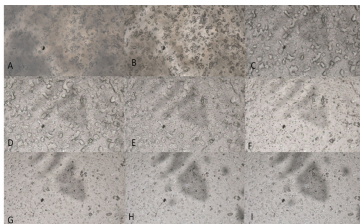
Figure 2. HSM analysis of films containing 19% malonic acid film at (A) 62^\circ\text{C} , (B) 65^\circ\text{C} , (C) 75^\circ\text{C} , (D) 76^\circ\text{C} , (E) 79^\circ\text{C} , (F) 83^\circ\text{C} , (G) 100^\circ\text{C} , cooling (H) 50^\circ\text{C} , reheating (I) 80^\circ\text{C} . Magnification of 100\times was used.
