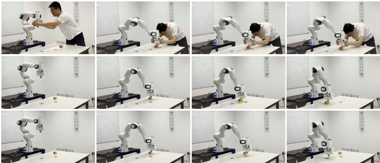
Fig. 18: Snapshots of the pushing task. First row illustrates the process of collecting a demonstration. Second and third rows show the robot executing the adapted trajectories obtained from our metric and the MAP metric, respectively.
