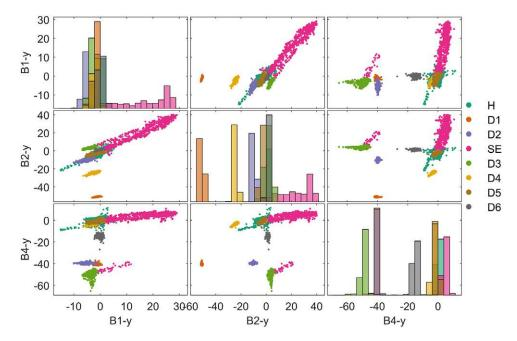
Figure 3. The standardized natural frequencies in the y-direction are plotted against each other. D1–D6 represent damage states, and H represents the normal condition data.
