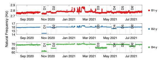
**Figure 2.** The features selected from the LUMO structure. The behavior of natural frequencies B1-y, B2-y, and B4-y throughout time. Each datapoint represents 10-minutes of measurements. D1-D6 highlight data collected during the damage states.
