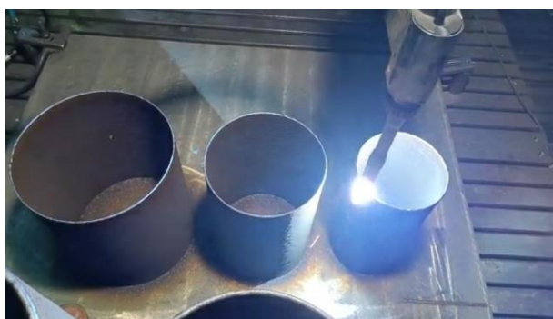
(a) WAAM CHS for compression tests
